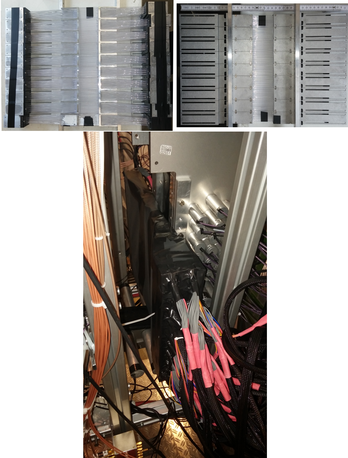
Figure 4.25.: Photographs of the final detector. The top row shows photographs of the fibres of the final detector set-up. The bottom picture shows the light tight ARGUS at its final position in front of the tagger.
