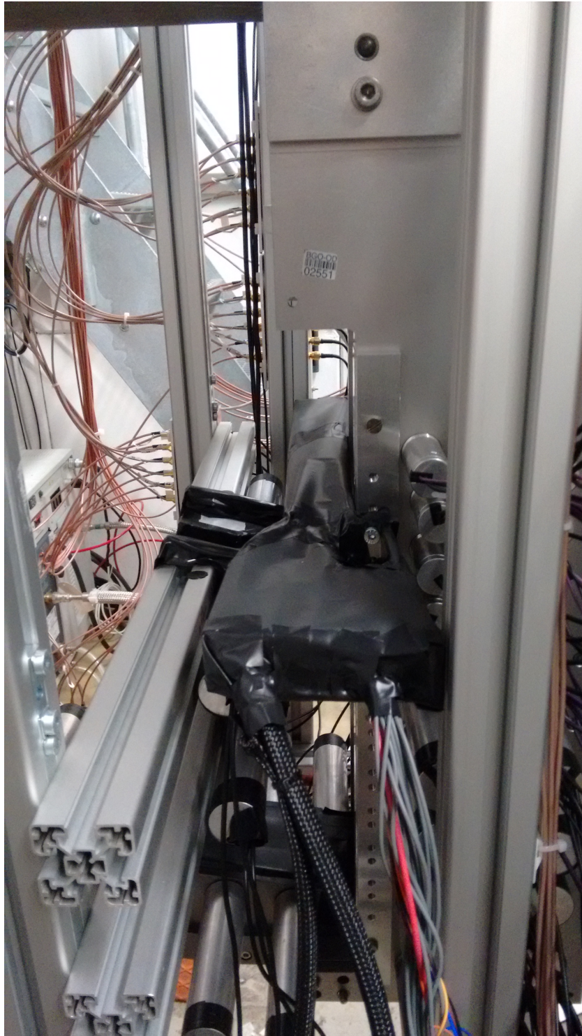
Figure 4.18.: Photograph of the prototype module with black foil around it, after being installed at the tagger. On the left the Møller polarimeter can be seen.
