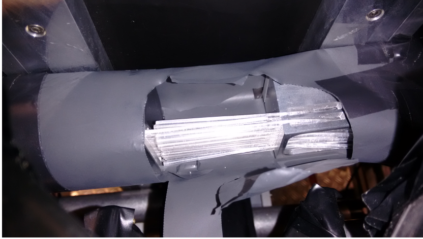
Figure 4.22.: Loose fibres after the first prototype test.
